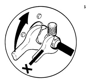
4. Using a marker or pen, mark a line lengthwise from the coupling union nut to the bulkhead. Then tighten the coupling and additional 1/4 turn. As the nut turns, the line will show when 1/4 turn is made.
