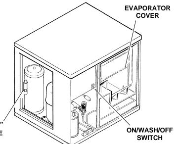
9. Observe water fill cycle: The water inlet solenoid valve OPENS, and water flows from the valve to the reservoir. The reservoir fills and excess water drains out the machine drain. At the end of the harvest cycle, the water inlet solenoid valve will close and the water fill cycle is complete. If the reservoir is not full, advance the shaft of the timer clockwise into a new harvest cycle; this opens the water valve again. The water pump will be pumping water over the evaporators.
